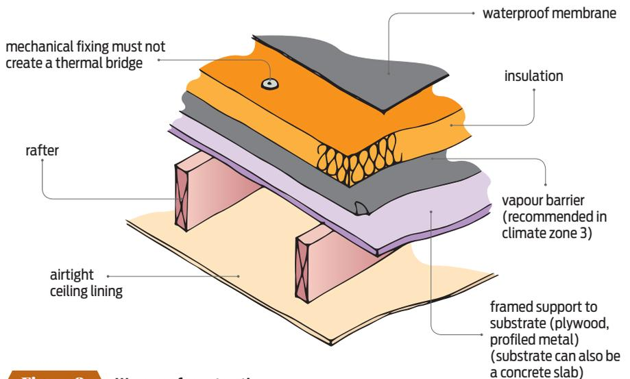
**Figure 2** Warm roof construction.
