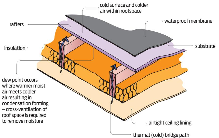
**Figure 1** Cold roof construction.
