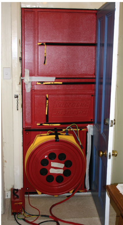
Figure 1: Blower door system used to measure airtightness.
