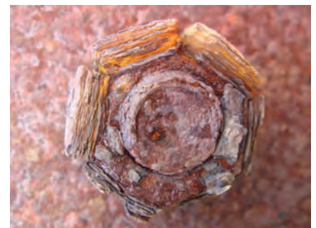
Figure 2: Mild steel nuts exposed at Judgeford (left) and Oteranga Bay (right) for 3 years.
