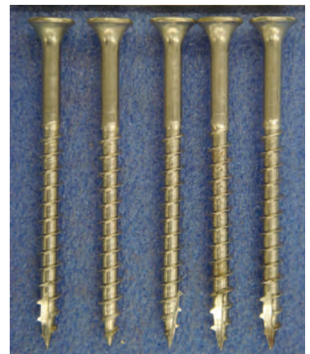
Figure 5: Stainless steel screws embedded into H4 ACQ treated timbers exposed at Oteranga Bay for 3 years. Limited rust was formed only on the head top.
