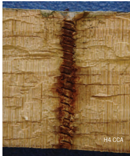
Figure 1: Iron stain formed by corrosion of zinc-coated screws in H4 CCA and H4 ACQ treated timbers exposed at Judgeford for 3 years.
