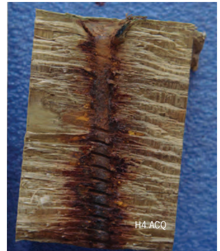
Figure 1: Iron stain formed by corrosion of zinc-coated screws in H4 CCA and H4 ACQ treated timbers exposed at Judgeford for 3 years.
