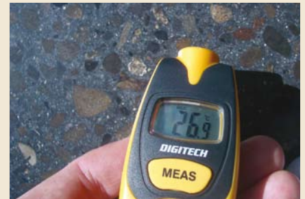
The darkened, polished concrete slab floor is an example of a material that has several functions – heat store, replacement floor covering and structural role
