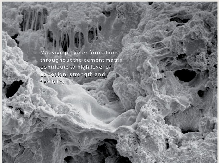
Massive polymer formations throughout the cement matrix contribute to high level of adhesion, strength and flexibility.
