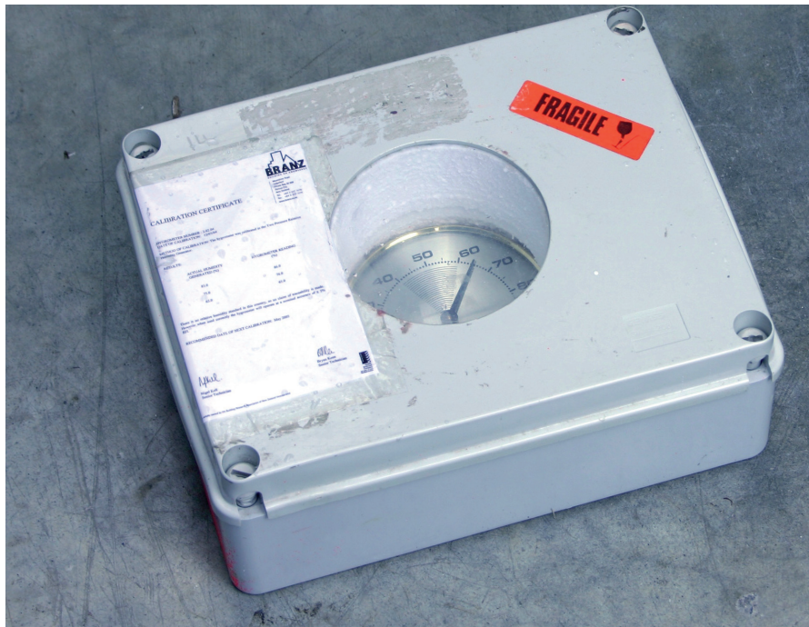
Figure 1: Flooring hygrometer installed on concrete slab.
