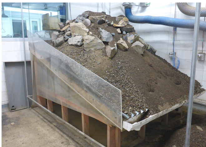
Figure 2: Tephra load during experiment (left) and the structural damage (right).
