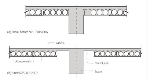
Figure 1: Details in NZS 3101 for hollowcore units adjacent to a beam.
