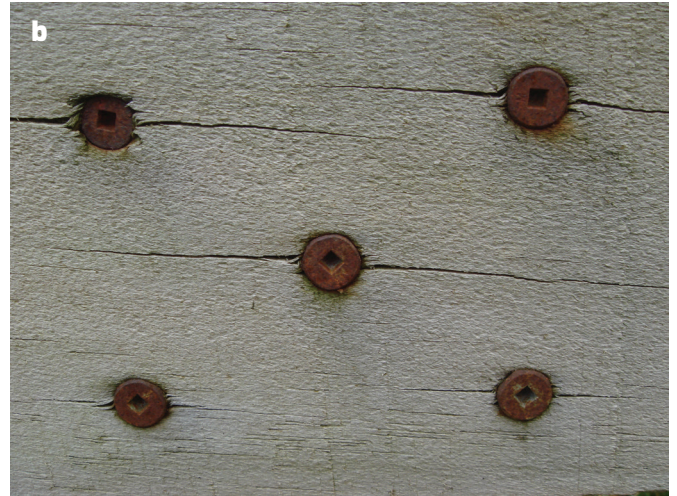
Figure 1: Durability of (a) hot-dip galvanised nail and (b) mechanically plated screws embedded into H4 copper azole and exposed at the BRANZ site in Judgeford for 3 years. Their zinc coating thicknesses are similar – approximately 50 µm.
