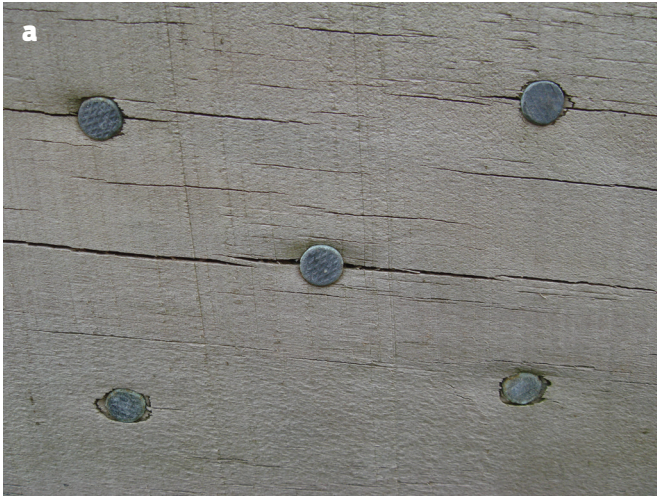
Figure 1: Durability of (a) hot-dip galvanised nail and (b) mechanically plated screws embedded into H4 copper azole and exposed at the BRANZ site in Judgeford for 3 years. Their zinc coating thicknesses are similar – approximately 50 µm.
