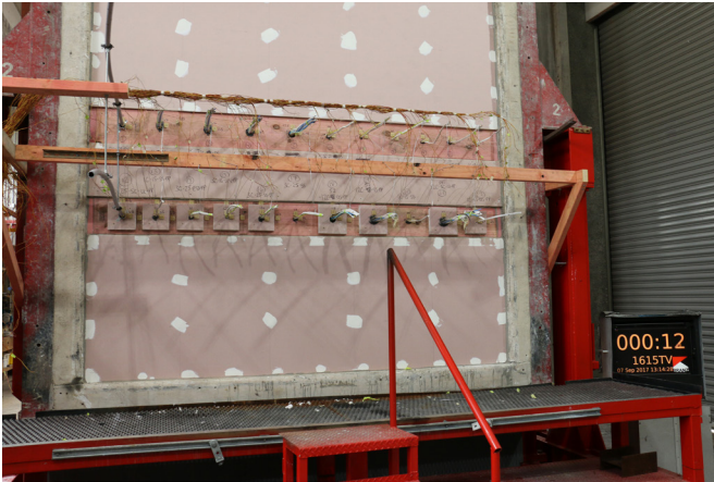
Figure 1: BRANZ fire research test investigates common firestopping construction details.
