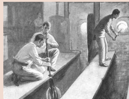
Blowing a glass cylinder around the early 1900s.
