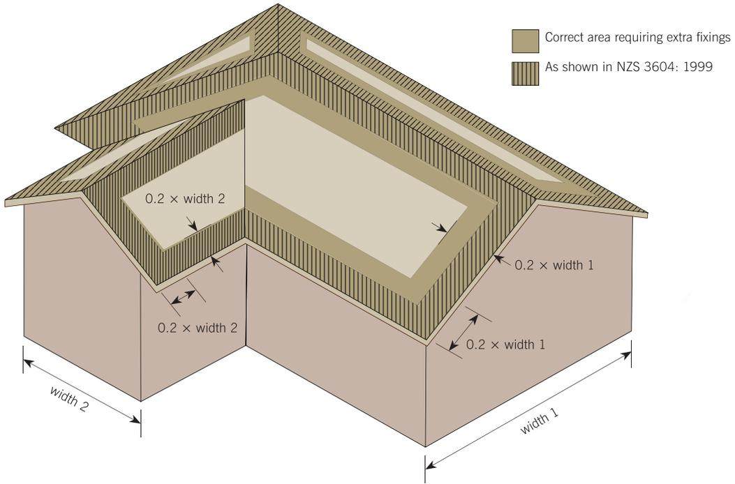
Figure 1: Hip and valley roof showing the areas that require extra purlin and batten fixings. (Adapted from NZS 3604: 1999, Figure 10.17.)
