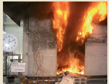
Flashover at the end of ISO 9705 test.
