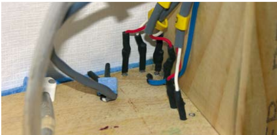
Figure 2: Moisture content measurement at a stud/dwang junction in experimental walls.
