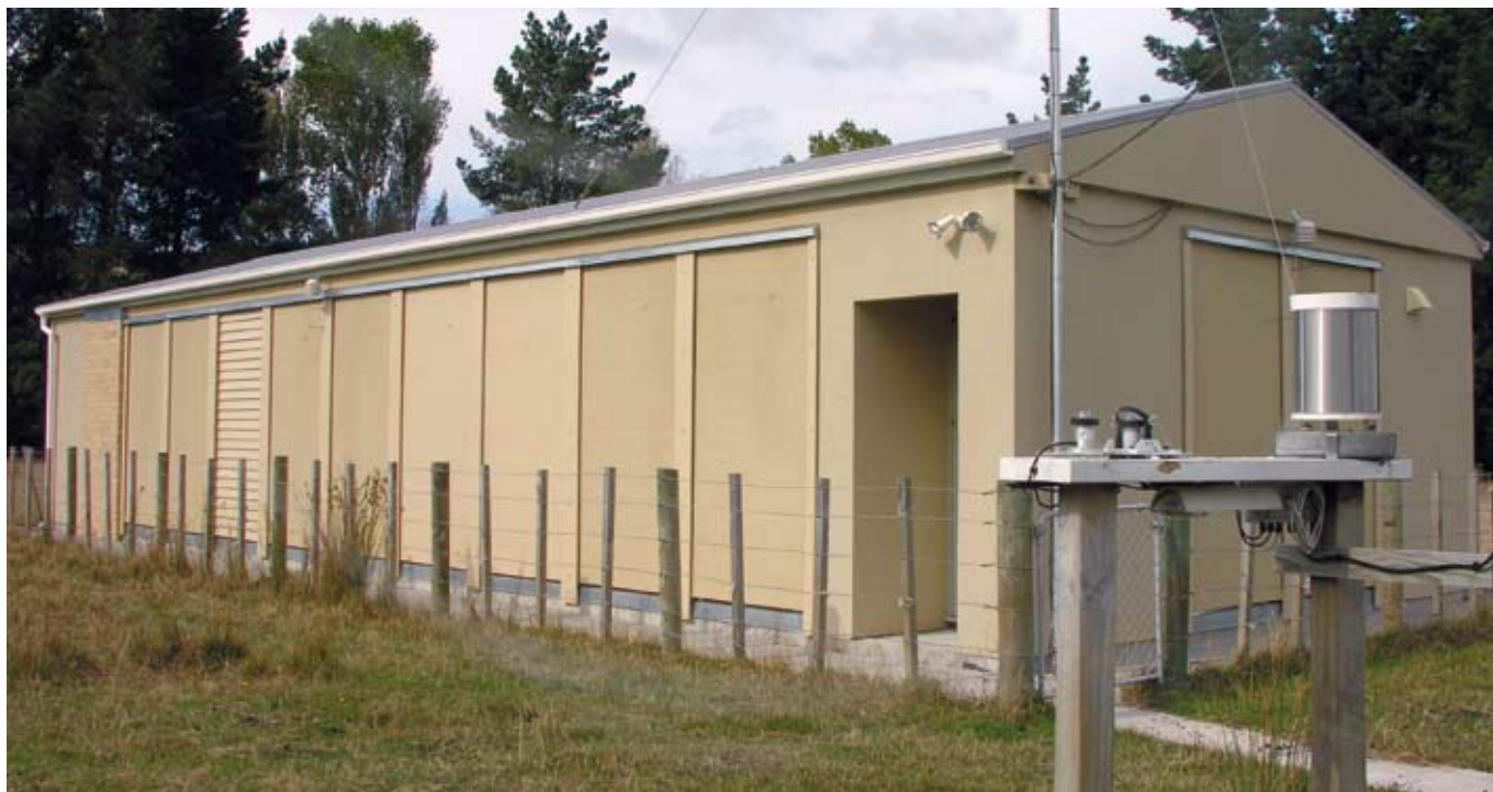
Figure 1: Experimental building at BRANZ showing the meteorological station in the foreground and experimental wall panels on the north and east faces.
