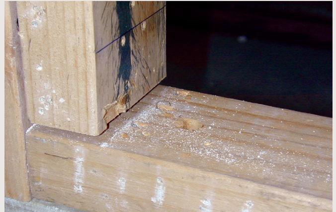
Damage to stud lift during laboratory testing.
