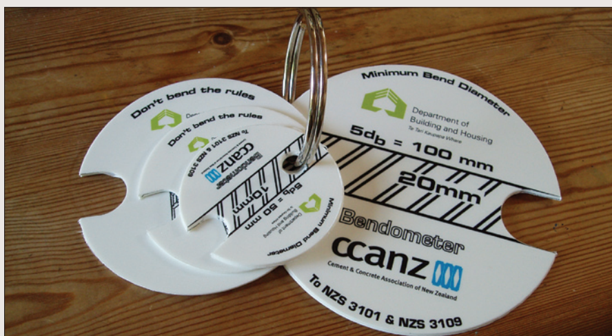
Figure 1: The Department of Building and Housing has a handy Bendometer tool for checking the radius of bends.
