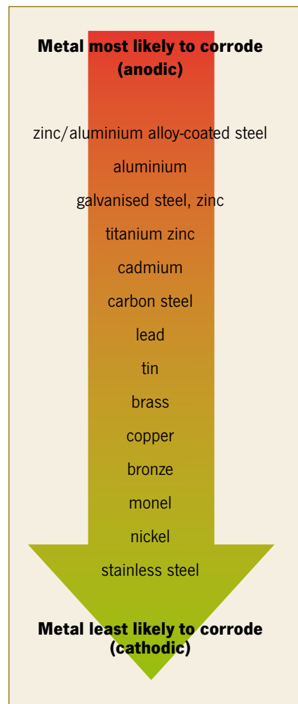
Figure 2: Galvanic series indicates the incompatibility of different metals.
