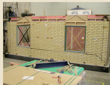
Figure 2: Clay brick veneer building after cyclic racking tests.
