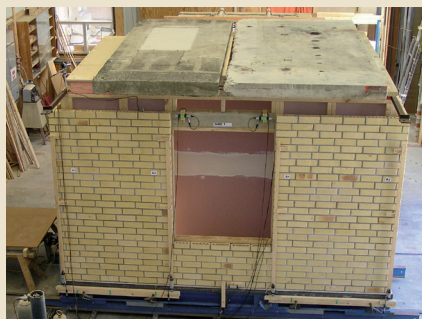
Figure 3: Building before shake table tests.
