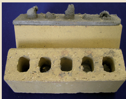
Figure 1: Clay bricks used showing mortar dowels.
