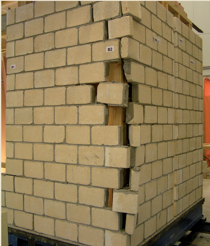
Figure 5: Damage to concrete brick veneer after extreme levels of shake table testing.
