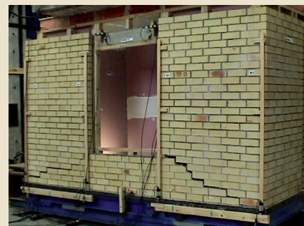
Figure 4: Building during shake table tests.
