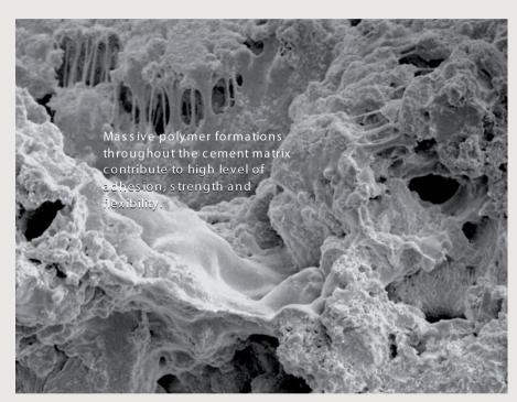
Figure 1: Massive polymer formations throughout the cement matrix contribute to high levels of adhesion, strength and flexibility. Width of field =  $69 \mu m$ .
