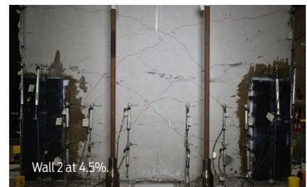
Figure 2: Out-of-plane failure and inadequate confinement of thin walls (courtesy of Zhibin Li).
