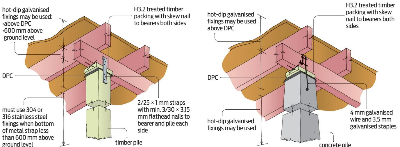
Figure 1: Jack and pack repair – timber pile (left) and concrete pile (right).
