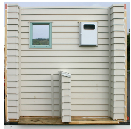
Figure 2: A typical E2/VM1 test specimen.
