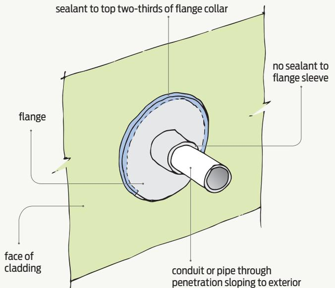
Note: Shaped packers sealed to cladding are required behind flange for profiled claddings.
