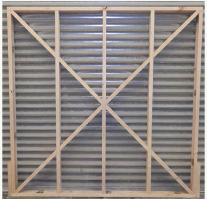
The Brace 3 specimen – double diagonal braces cut between studs.
