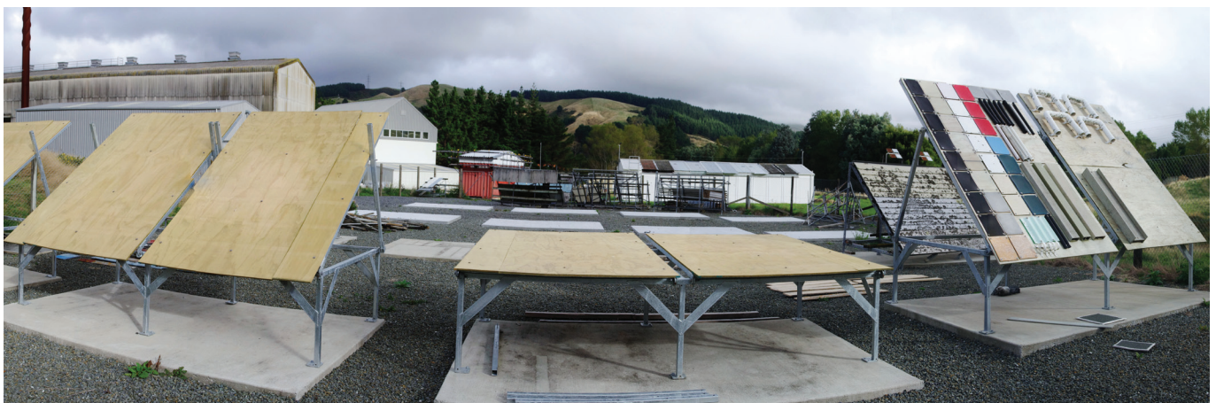
Building products on the upgraded exposure site racks at BRANZ include claddings, coatings, pipes, flashings, membranes, roofing products and even different nails and screws in treated timbers.
