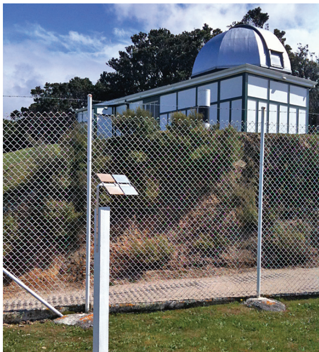
An exposure rack carrying mild and galvanised steel panels installed at MetService's meteorological station at Kelburn, Wellington.
