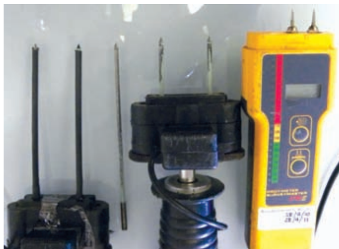
A range of resistance meter pins. From left deep wall pins with additional shrink wrap insulation, single pin with worn insulation over most of shank, short sliding hammer pins with compromised insulation and fixed uninsulated pins.
