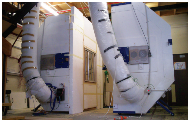
The BRANZ Guarded Hot Box open with the aluminium framed secondary glazing installed in the window.
