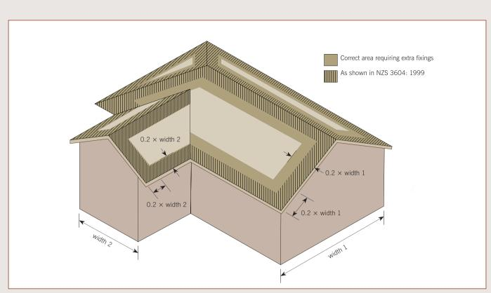
Figure 1: Hip and valley roof showing the areas that require extra purlin and batten fixings. (Adapted from NZS 3604: 1999, Figure 10.17.)
